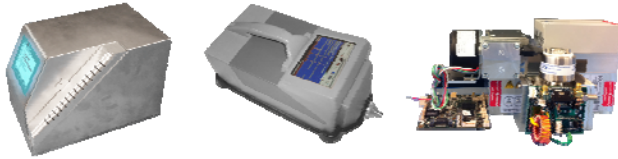
Figure 1 – Photographs of 3 variants of 1 st Detect miniature mass spectrometer including bench-top (left), handheld (center), and sub-component (right)
