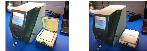
Figure 5 – photograph of MCD with evacuated desorber explosives sampler
