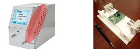
Figure 7 – photograph of pre-concentrator (right) and external location for easy maintenance
