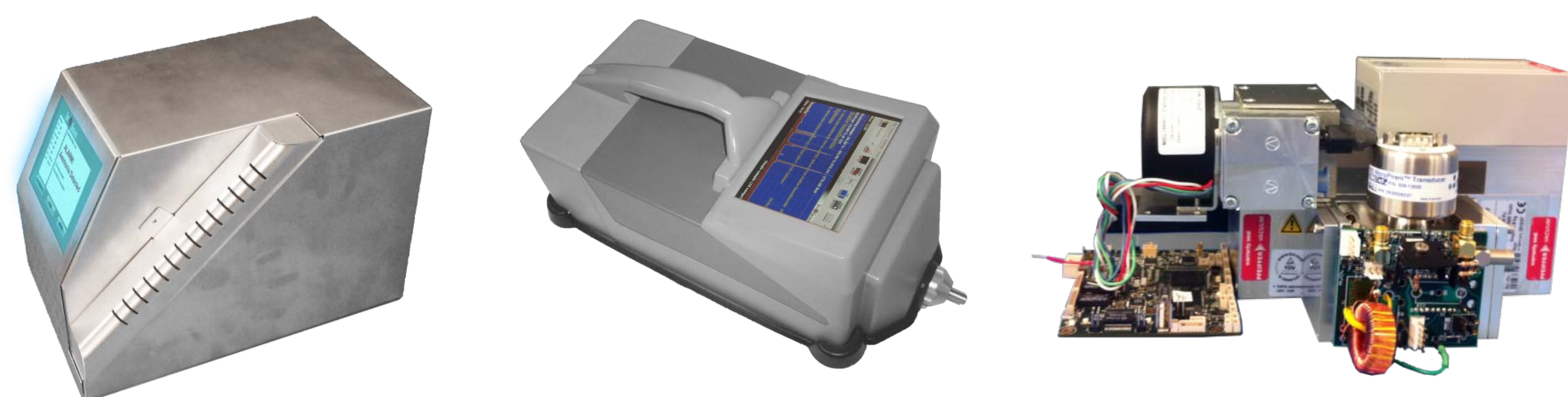
Figure X – Photographs of 3 variants of 1 st Detect miniature mass spectrometer including bench-top (left), handheld (center), and sub-component (right)
